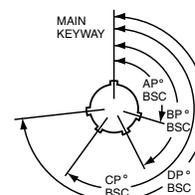
A plug with a given rotation letter will mate with a receptacle with the same rotation letter. The angles for a given connector are the same whether it contains pins or sockets. Inserts are not rotated in conjunction with the master key/keyway.
