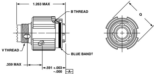
† Blue band indicates rear release contact retention system
