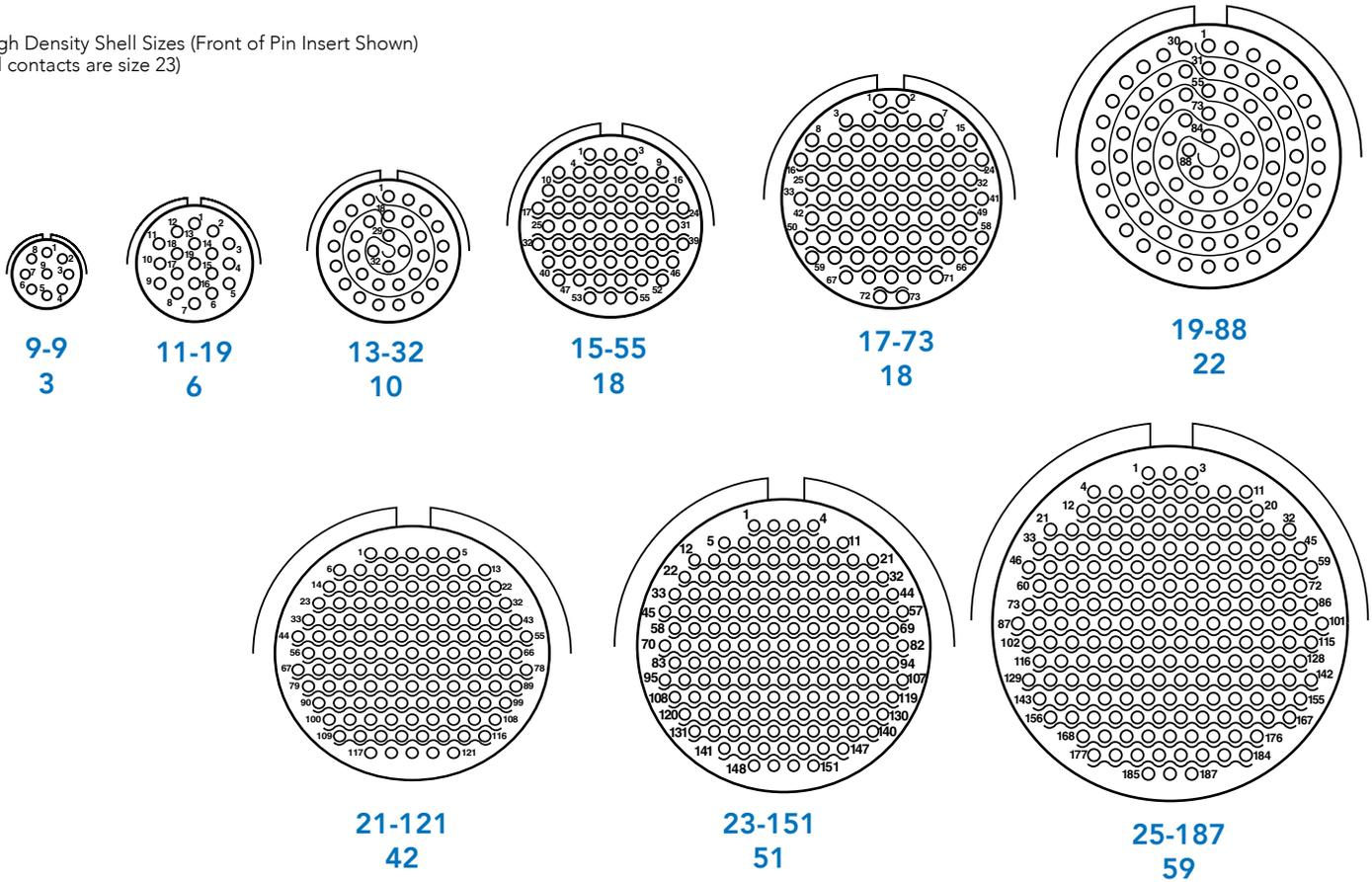
Increased number of contacts in HD38999 insert pattern compared to Standard 38999\*contact density of same shell size.
