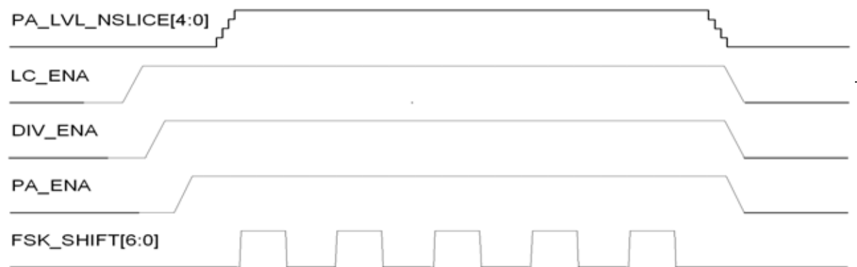
Figure 13.2. FSK Timing Example
