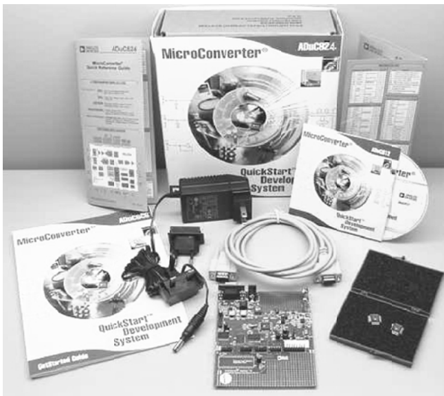
Figure 54. Components of the QuickStart Development System
