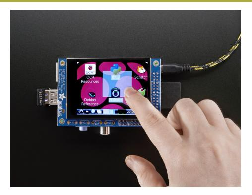
The nifty thing about capacitive touch screens is that they **do not require calibration!** The calibration is done 'in chip' on the screen itself. However, we still do need to tell the Pi how to read the capacitive chip.
