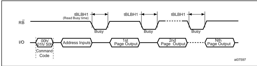
**Figure 13. Sequential row read block diagrams**
