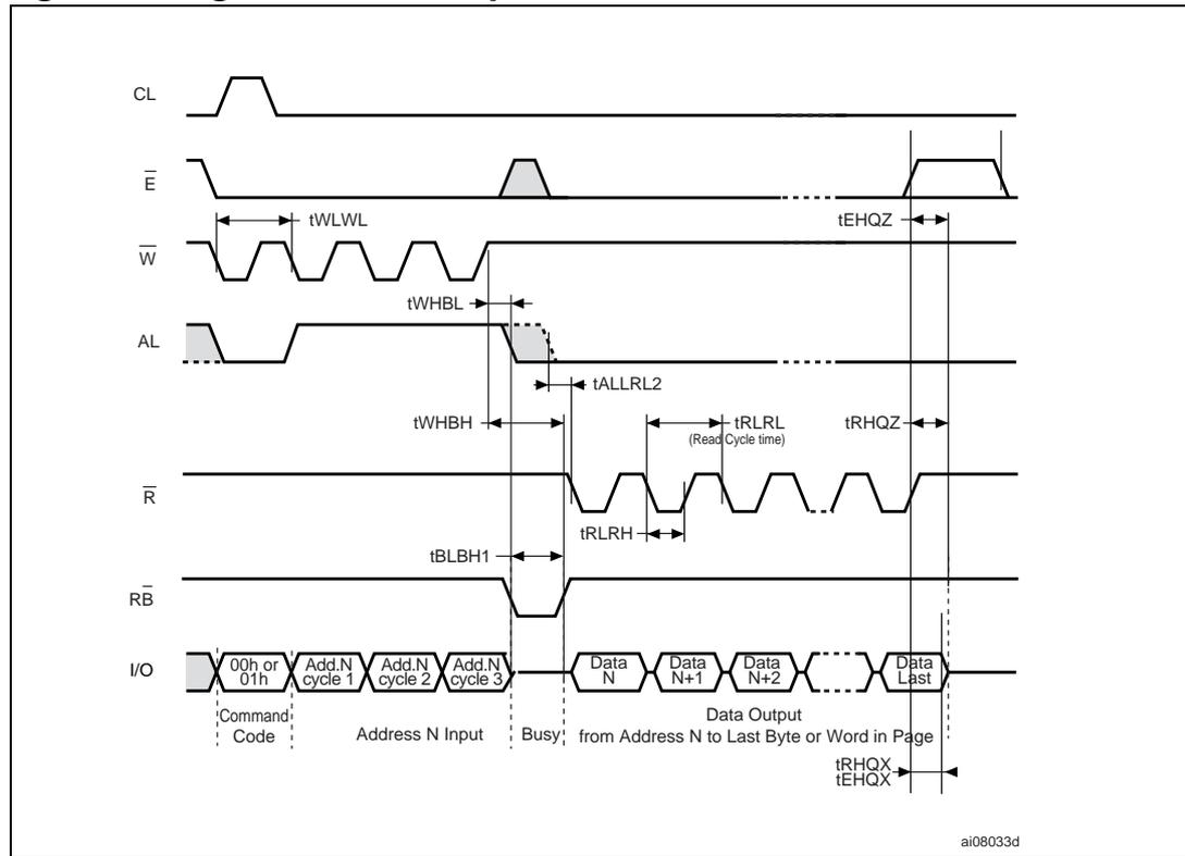
Figure 28. Read C operation, one page AC waveform
