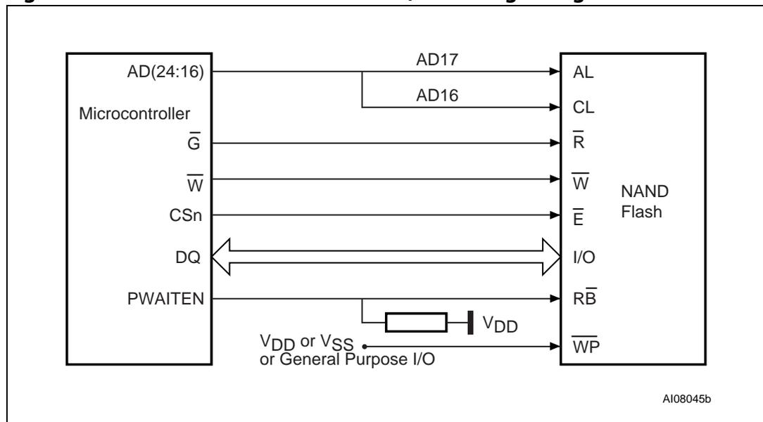
Figure 39. Connection to microcontroller, with glue logic
