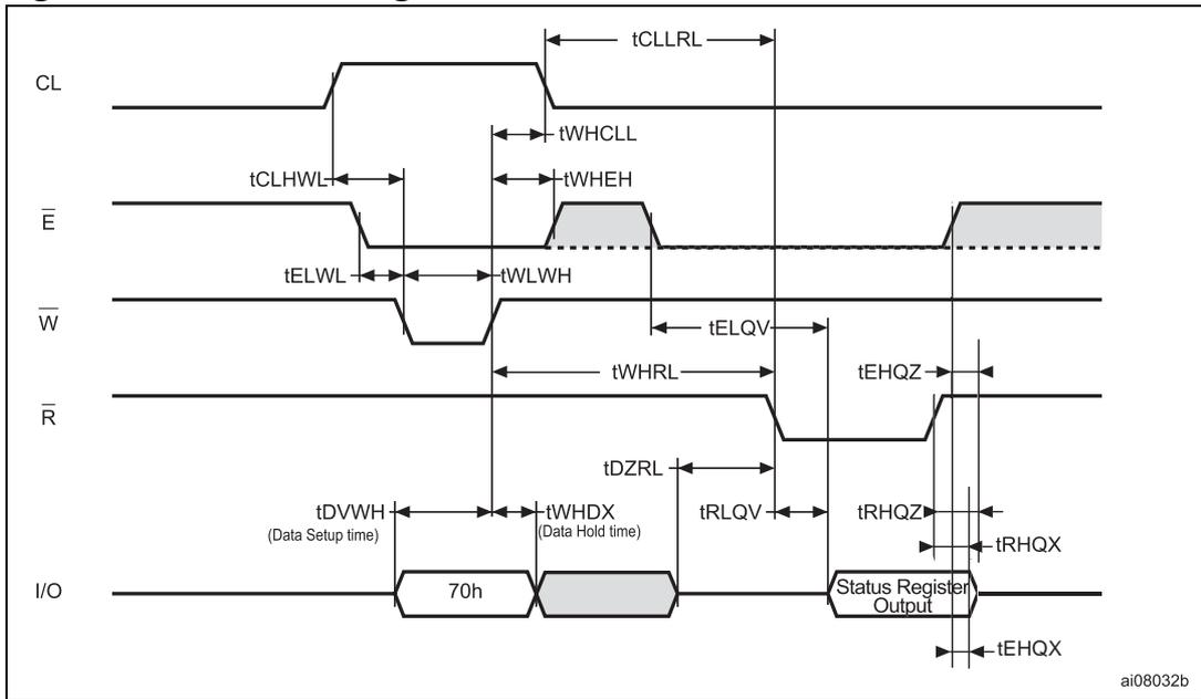
**Figure 26. Read electronic signature AC waveform**
