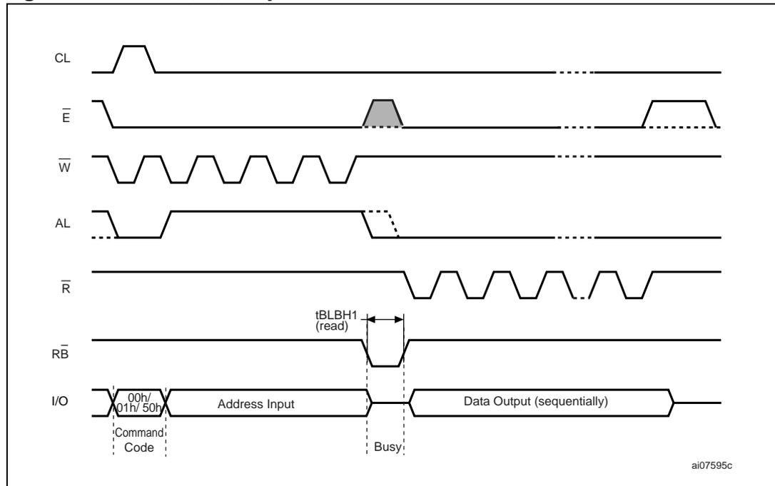
**Figure 11. Read block diagrams**
