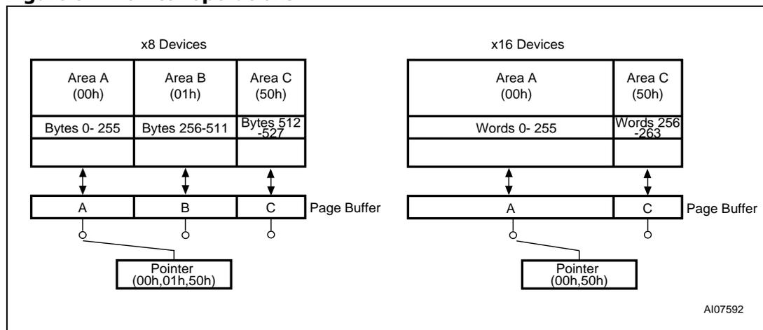
**Figure 9. Pointer operations for programming**
