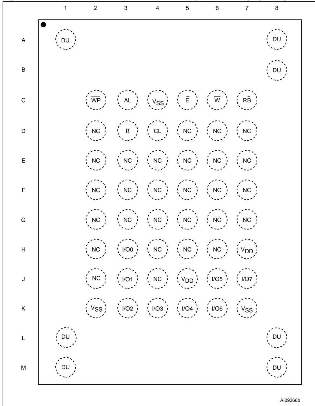
Figure 6. VFBGA55 connections, x16 devices (top view through package)
