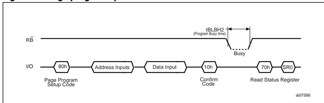
1. Before starting a page program operation a pointer operation can be performed. Refer to [Section 6.1: Pointer operations](#) for details.
