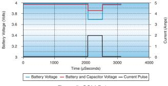
Figure 5. GSM Pulse
