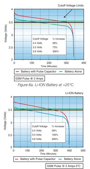
Figure 6b. Li-ION Battery at +0°C
