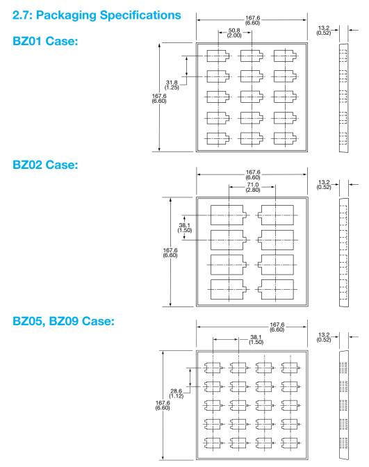
This specification applies when our electrochemical supercapacitors are packed using a 165mm by 165mm container. The parts are held in place by a 166mm by 166mm lid.
