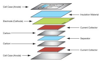
Electrons are relatively fast moving and therefore transfer charge "instantly." However, ions have to move relatively slowly from anode to cathode, and hence a finite time is needed to establish the full nominal capacitance of the device. This nominal capacitance is normally measured at 1 second.
