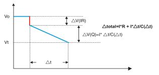
Figure 4. Voltage-time relation of capacitor unit
