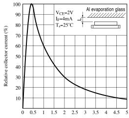
Distance between sensor and Aluminum evaporation glass L (mm)
