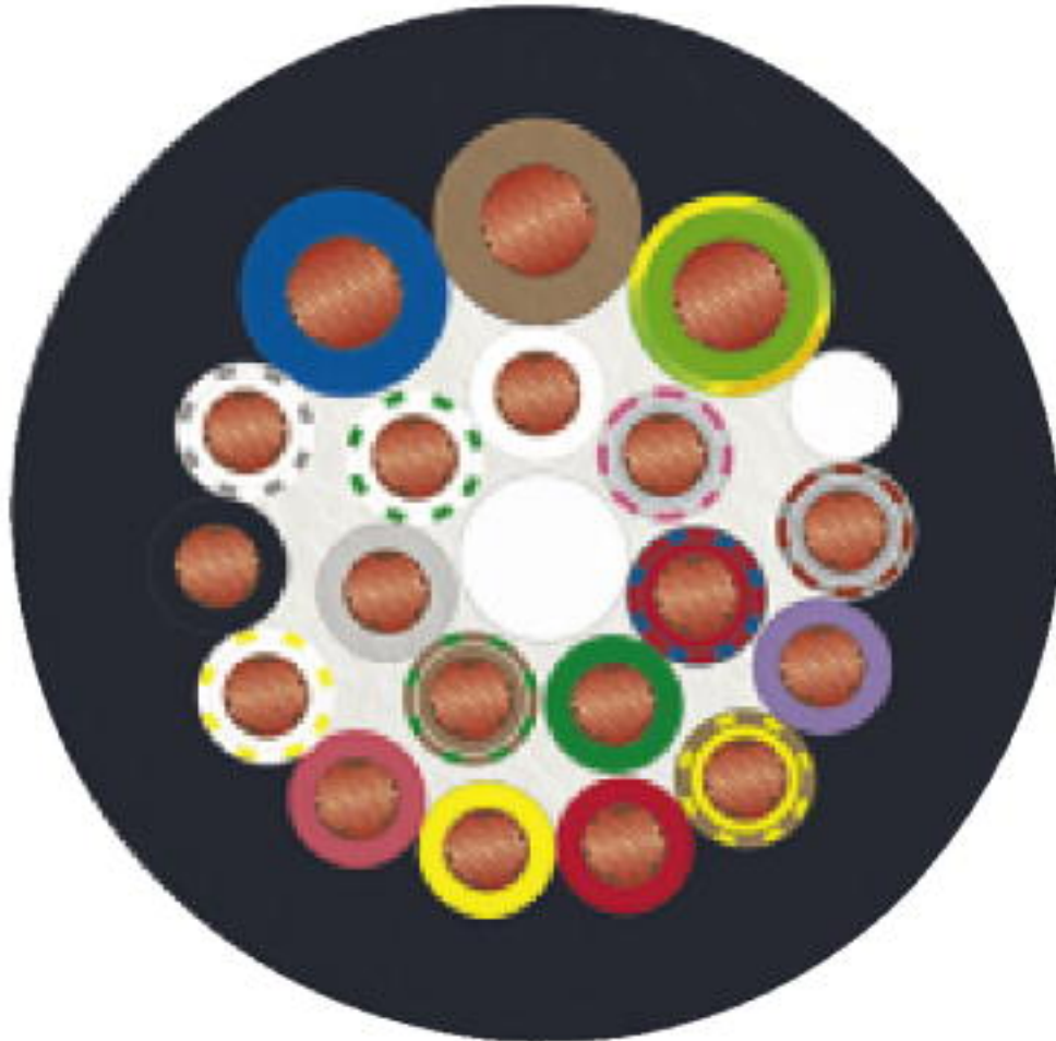
Cable cross section
