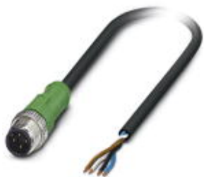
Sensor/actuator cable, 4-position, PVC, black RAL 9005, Plug straight M12, A - standard, on free cable end, cable length: 5 m
