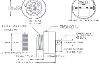
NOTE A: TERMINALS-032 BRASS TIN PLATED, TAPPED FOR #6-32 SCREW. TWO #6-32 NICKEL PLATED BRASS SCREWS INCLUBED. WILL ACCEPT 1/4\* QUICK CONNECT.
