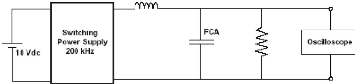
In the above circuit, one 1  $\mu\text{F}$  FCA capacitor results in the same ripple reduction performance as a 10  $\mu\text{F}$  tantalum capacitor at 200 kHz. With a 1  $\mu\text{F}$  tantalum capacitor in the circuit the measured ripple voltage was 70 mVpp, and with a 10  $\mu\text{F}$  tantalum or a 1  $\mu\text{F}$  FCA capacitor the ripple voltage was 8 mVpp.
