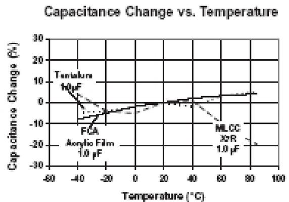
Type FCA capacitors have very low e.s.r. and stable capacitance vs. temperature.
