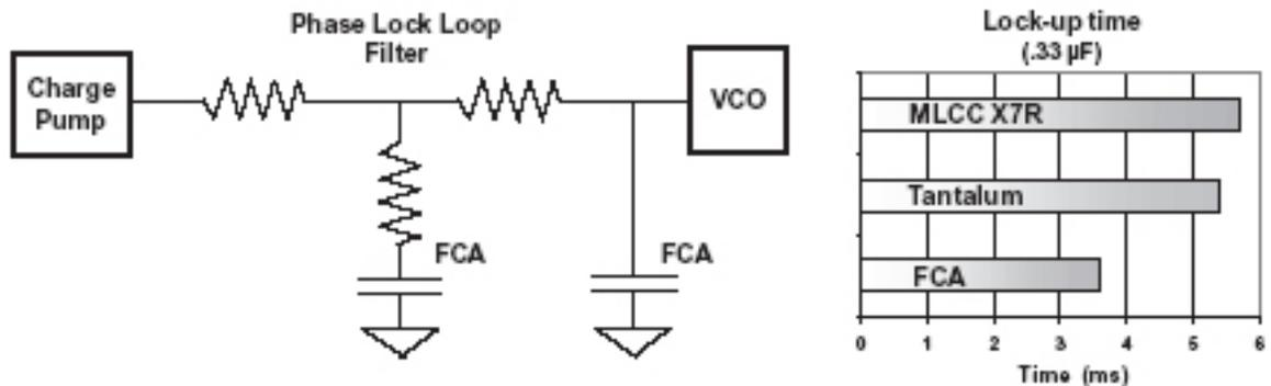
FCA surface mount film capacitors have advantages over tantalum and ceramic capacitors in PLL circuits. There are no piezoelectric effects to create noise, they are not polarized, and they result in faster signal lock-up time.
