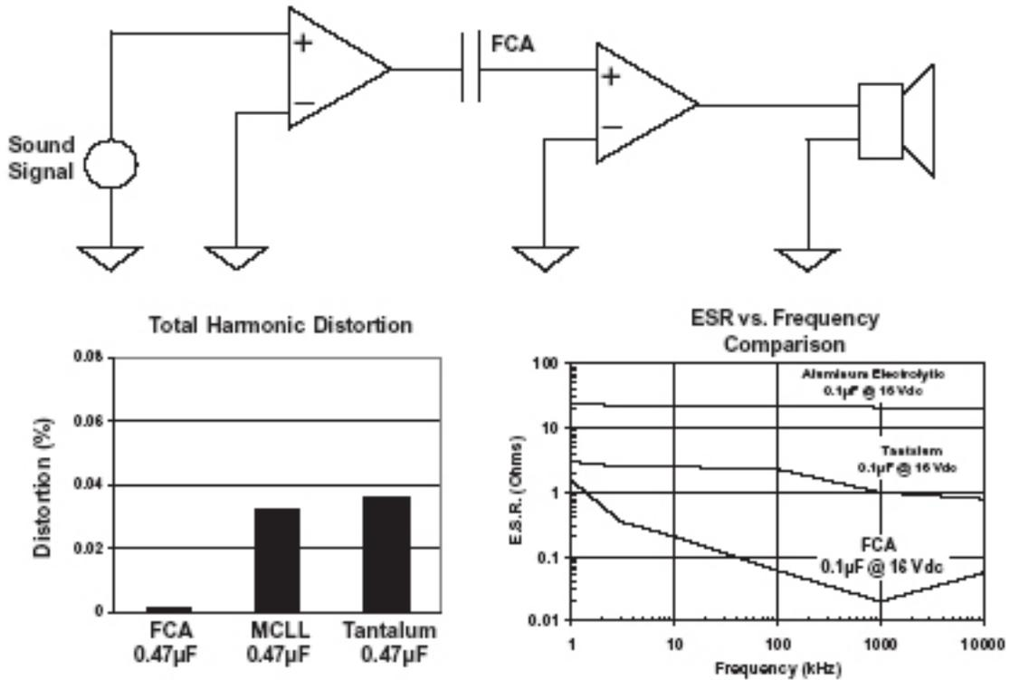
Using FCA capacitors in audio circuits can result in lower sound distortion. The low e.s.r., the absence of piezoelectric effects, and the non polar nature of the capacitor will eliminate sources of distortion in your audio circuits.
