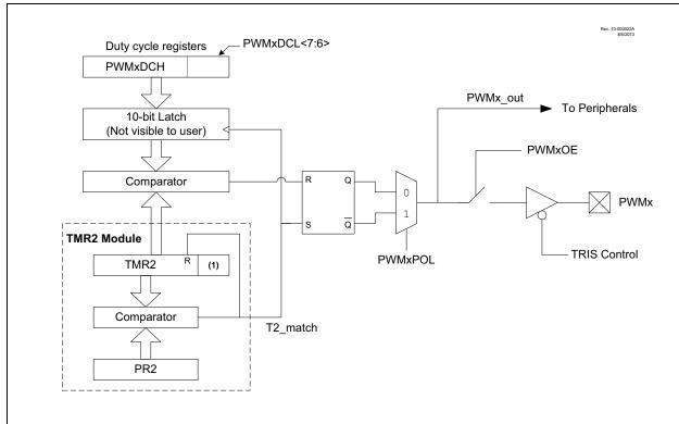
**Note 1:** 8-bit timer is concatenated with two bits generated by Fosc or two bits of the internal prescaler to create 10-bit time-base.
