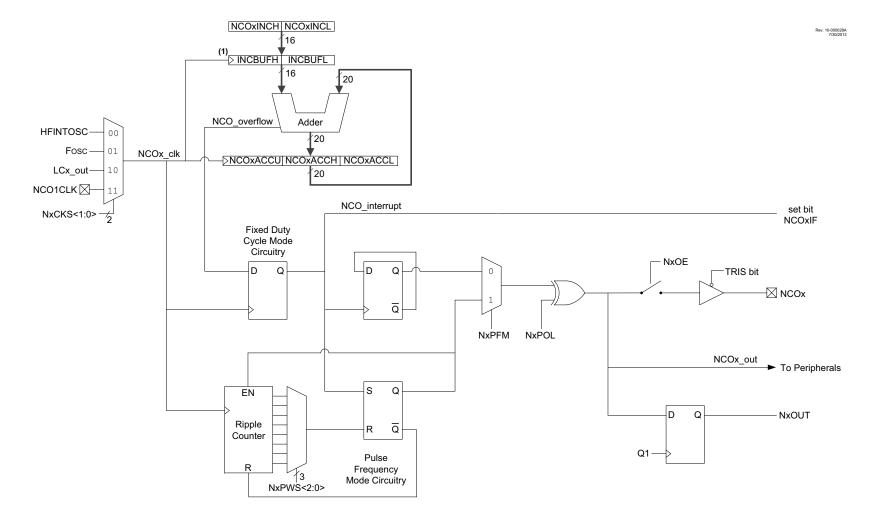
Note 1: The increment registers are double-buffered to allow for value changes to be made without first disabling the NCO module. The full increment value is loaded into the buffer registers on the second rising edge of the NCOx\_clk signal that occurs immediately after a write to NCOxINCL register. The buffers are not user-accessible and are shown here for reference.
