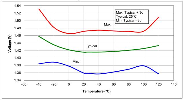
FIGURE 28-43: BROWN-OUT RESET VOLTAGE, BORV = 1, PIC12LF1501 ONLY
