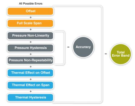
Figure 1. TEB Components for TruStability® Board Mount Pressure Sensors
