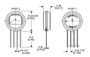
**SIP SN:** Manifold mount, inner diameter seal
