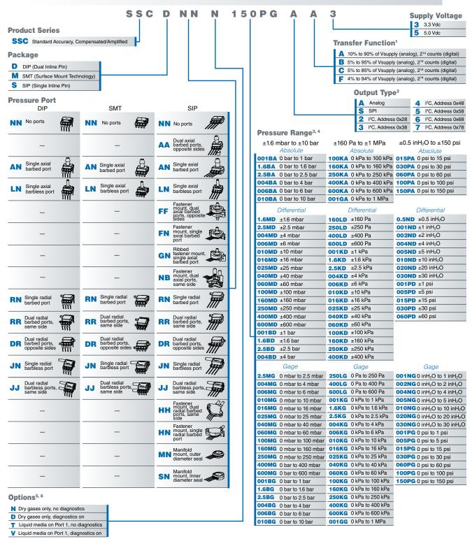
The transfer function limits define the output of the sensor at a given pressure input. By specifying Pmin. and Pmax., the output at Pmin. and Pmax., the complete transfer function of the sensor is defined. See the graphical representations of the transfer function in Figure 2. For other available transfer functions contact Honeywell Customer Service. <sup>2</sup>SPI output function is not available in SIP package.
