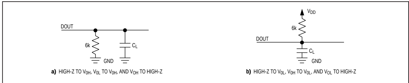
Figure 1. Load Circuits for Enable and Disable Time
