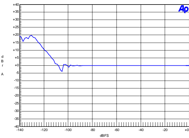
Figure 51. 96 kHz, Fade-to-Noise Linearity
