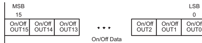
Figure 8. On/Off Data Format
