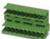
Header, Nominal current: 10 A, Rated voltage (III/2): 320 V, Number of positions: 5, Pitch: 5 mm, Color: green, Contact surface: Tin, Mounting: Wave soldering, Can be aligned! Mounting flange: Order No. 1736771, 1736768. In combination with MVSTB or FKCV plug components, both an MVSTBW (or FKCVW) and an MVSTBR plug (or FKCVR) must be used. Combination with TMSTBP plug components is not possible!
