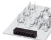
Header, Nominal current: 12 A, Rated voltage (III/2): 320 V, Number of positions: 5, Pitch: 5 mm, Color: black, Contact surface: Tin, Mounting: THR soldering, User information and design recommendations for through hole reflow technology can be found under "Downloads"
