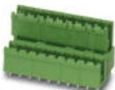
Header, Nominal current: 10 A, Rated voltage (III/2): 320 V, Number of positions: 5, Pitch: 5 mm, Color: green, Contact surface: Tin, Mounting: Wave soldering, Can be aligned! Mounting flange: Order No. 1836477, 1836480. In combination with MVSTB or FKCV plug components, both an MVSTBW (or FKCVW) and an MVSTBR plug (or FKCVR) must be used. Combination with TMSTBP plug components is not possible!
