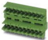
Header, Nominal current: 10 A, Rated voltage (III/2): 320 V, Number of positions: 5, Pitch: 5 mm, Color: green, Contact surface: Tin, Mounting: Wave soldering, The article can be aligned to create different nos. of positions! In combination with MVSTB or FKCV plug components, both an MVSTBW (or FKCVW) and an MVSTBR plug (or FKCVR) must be used. Combination with TMSTBP plug components is not possible!
