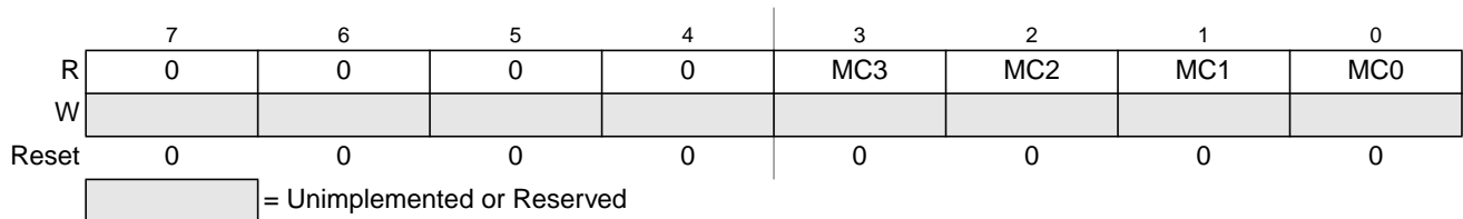
Figure 6-12. Debug Match Flag Register (DBGMFR)
