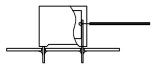
Temperature monitored inside the capacitor.
