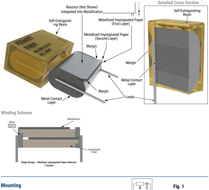
RC units are mounted in parallel with the contacts to be protected or in parallel with the inductive load (Fig. 1 and Fig. 2). RC units are generally mounted in parallel with the contacts to suppress radio interferences (Fig. 1).
