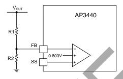
Figure 2. Voltage Divider Circuit
