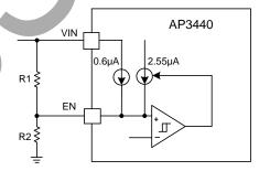
Figure 1. Adjustable Under Voltage Lock Out
