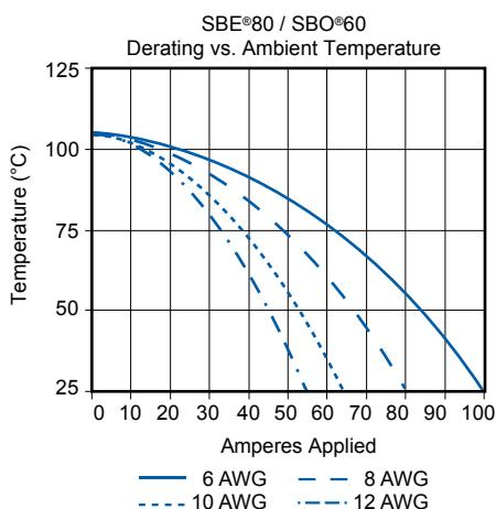
NOTE: Temperature rise charts are based on a 25°C ambient temperature.
