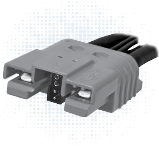
SBE® and SBO® connectors build on the capability of the two pole SB® connectors by offering up to 8 auxiliary power / signal contacts along with an IEC 60950 touch safe housing. The center of the main connector features a connector holder for either: two PP15-45, two PPMX, or APP's innovative 1x4 auxiliary connector.
