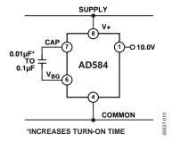
Figure 9. Additional Noise Filtering with an External Capacitor
