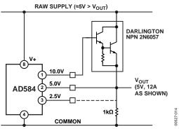
Figure 13. NPN Output Current Booster
