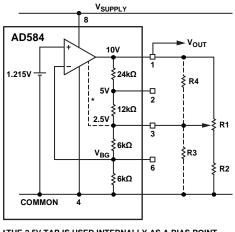
\*THE 2.5V TAP IS USED INTERNALLY AS A BIAS POINT AND SHOULD NOT BE CHANGED BY MORE THAN 100mV IN ANY TRIM CONFIGURATION.
