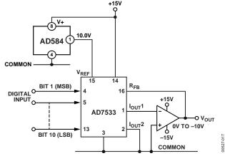
Figure 16. Low Power 10-Bit CMOS DAC Application
