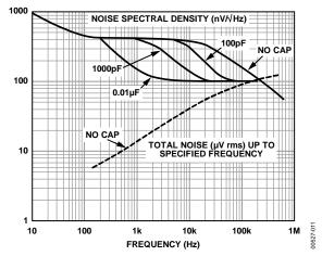
Figure 10. Spectral Noise Density and Total RMS Noise vs. Frequency
