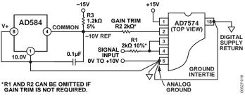
Figure 17. AD584 as -10 V Reference for CMOS ADC
