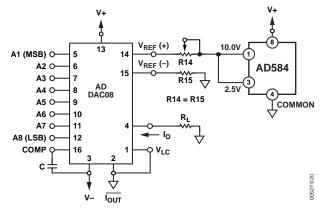
Figure 18. Current Output, 8-Bit Digital-to-Analog Configuration
