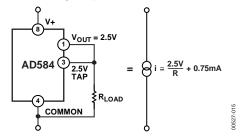
Figure 14. A Two-Component Precision Current Limiter
