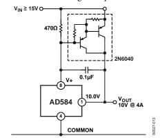
Figure 12. High Current Precision Supply
