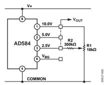
Figure 4. Output Trimming
