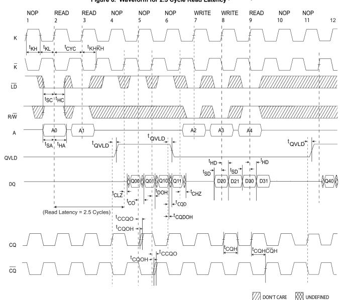
**Read/Write/Deselect Sequence** Figure 6. Waveform for 2.5 Cycle Read Latency [37, 38, 39]
