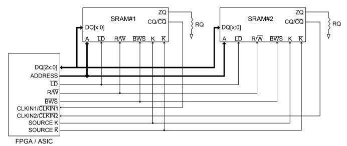
Figure 2. Application Example (Width Expansion)
