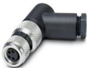
Connector, Universal, 4-position, Socket angled M8, Coding: A, Screw connection, knurl material: Nickel-plated brass, external cable diameter 3.5 mm ... 5 mm
