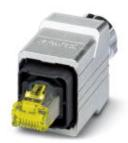
RJ45 connector, IP67, with push/pull interlocking (version 14), metal housing, for 10 Gbps, for AWG 24 ... 27 stranded conductors
