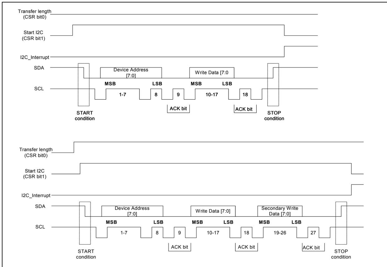
**Figure 9: I<sup>2</sup>C Write Mode Operation**
