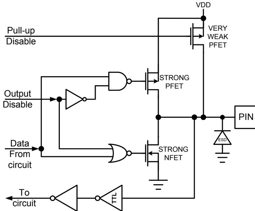
Figure 29: Digital I/O with Pull Up Circuit
