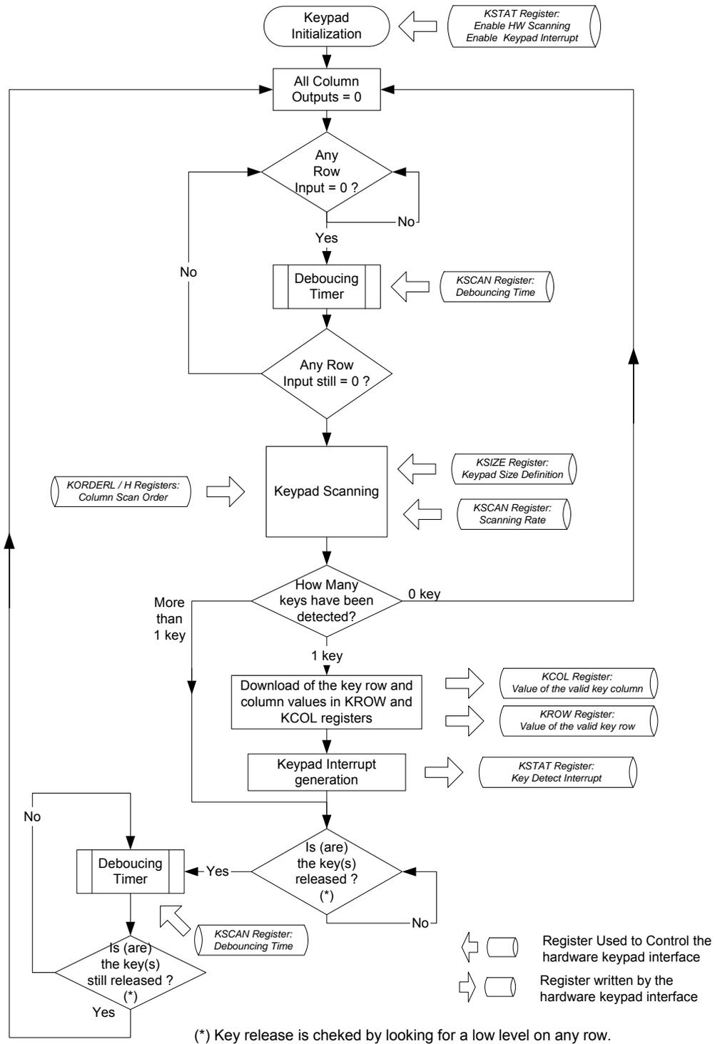
Figure 12: Keypad Interface Flow Chart
