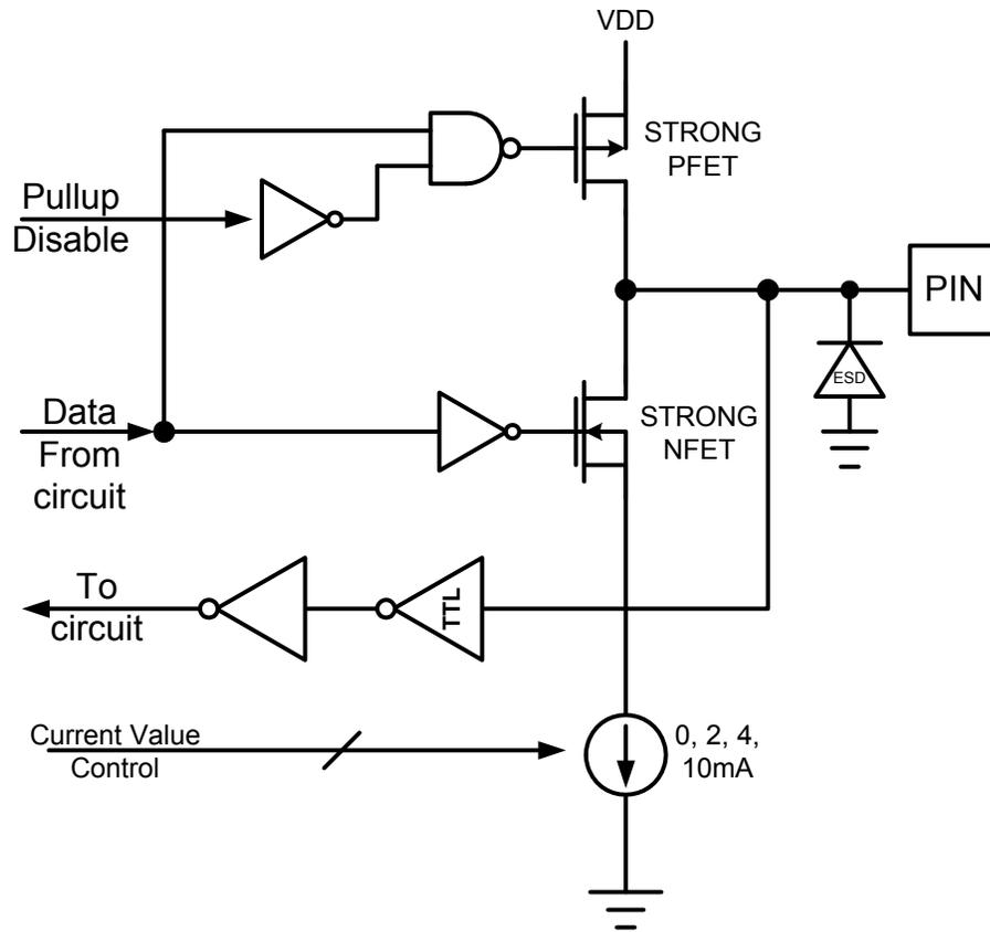
Figure 34: LED Circuit
