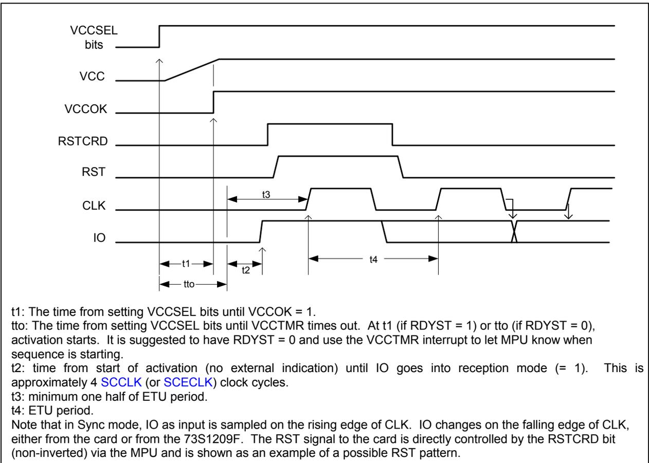
**Figure 19: Synchronous Activation**
