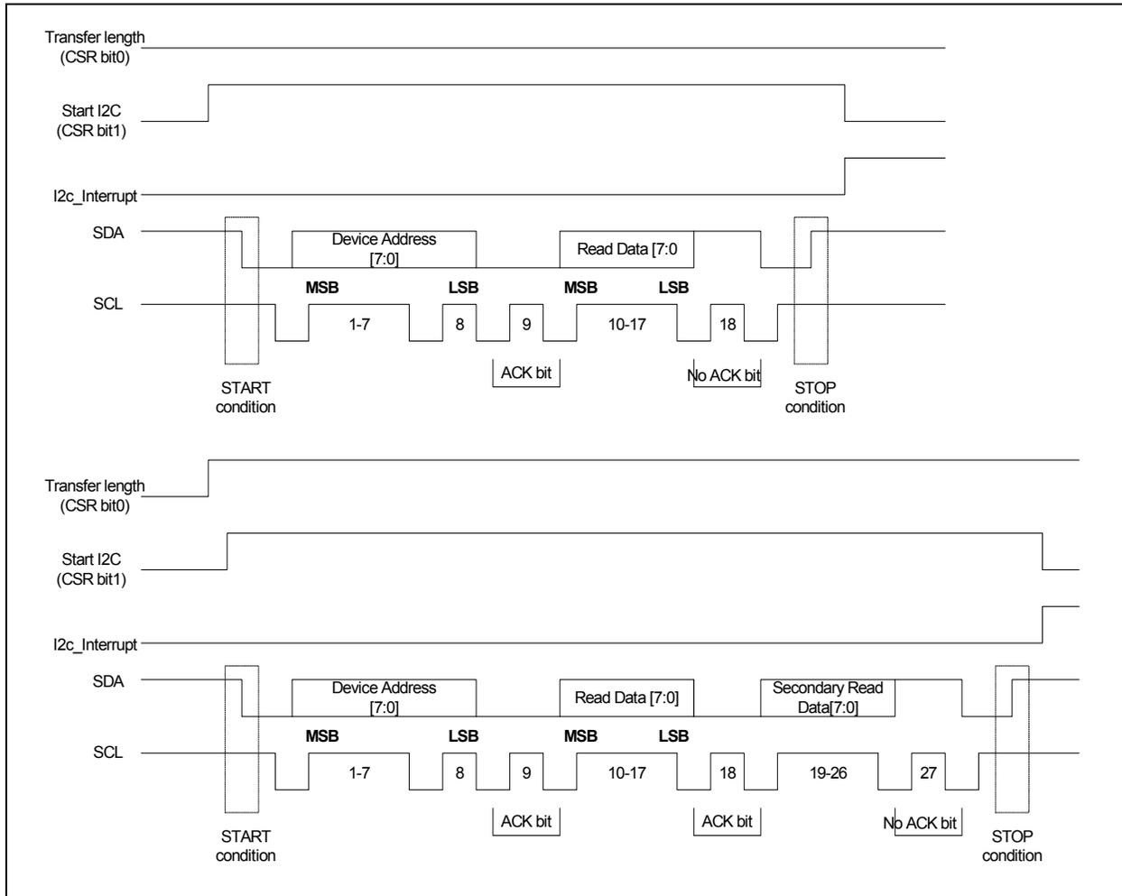
Figure 10: I<sup>2</sup>C Read Operation
