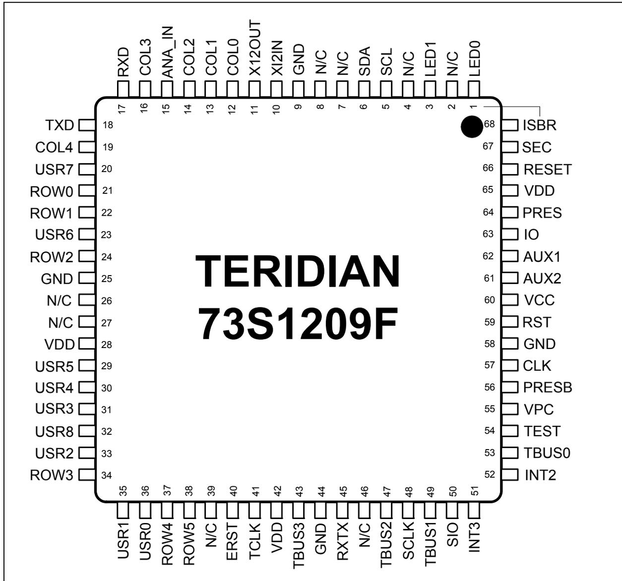
Figure 41: 73S1209F Pinout
