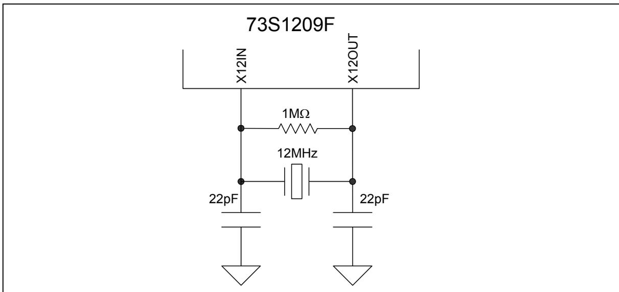
Note: The crystal should be placed as close as possible to the IC, and vias should be avoided.
