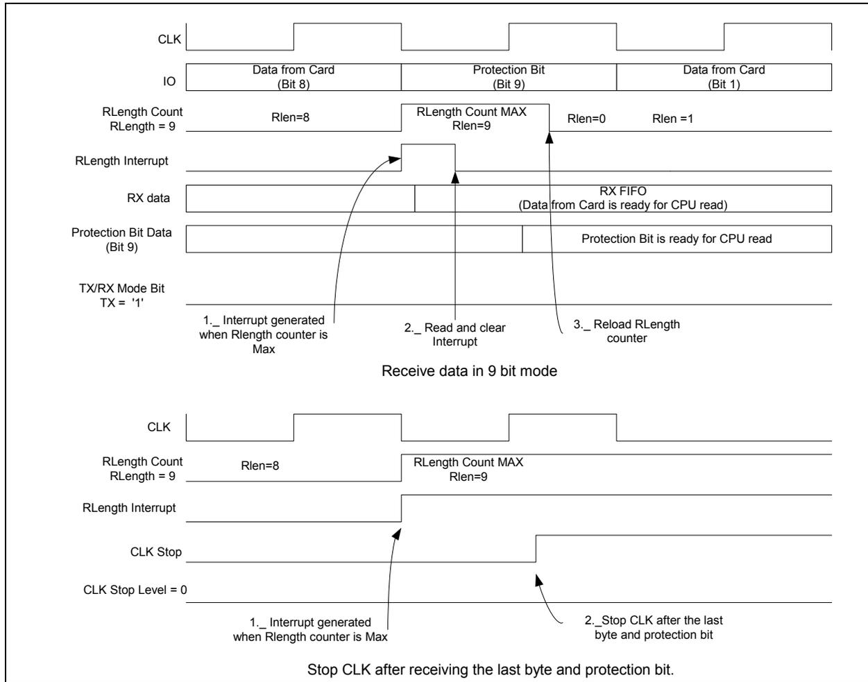
**Figure 23: Operation of 9-bit Mode in Sync Mode**
