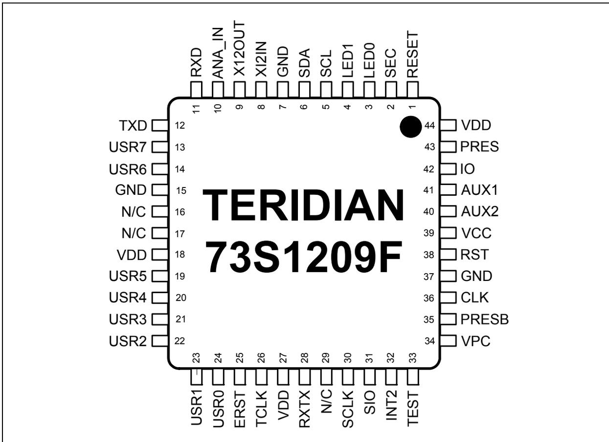
Figure 42: 73S1209F Pinout
