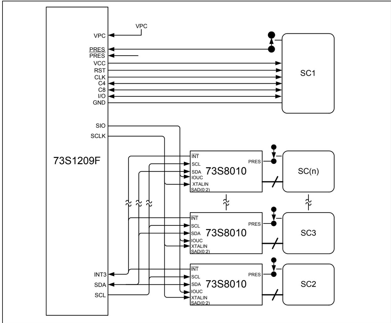
Figure 14: External Smart Card Interface Block Diagram
