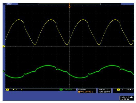
Figure 11. Reverse Phase Dimming: Rectified Input Voltage (Top) and Input Current (Bottom) - Full
