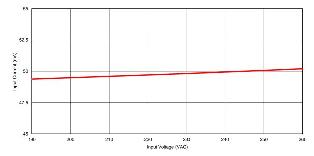
Figure 3. Input (Linear Regulator) Current Versus Input Voltage
