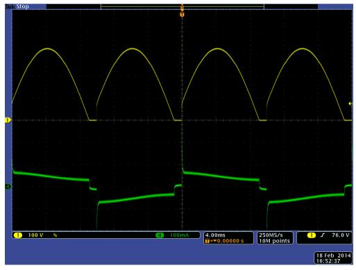
Figure 8. Forward Phase Triac Dimming: Rectified Input Voltage (Top) and Input Current (Bottom) - Full
