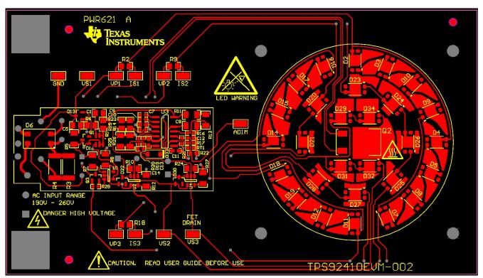
Figure 15. Top Layer and Top Overlay (Top View)
