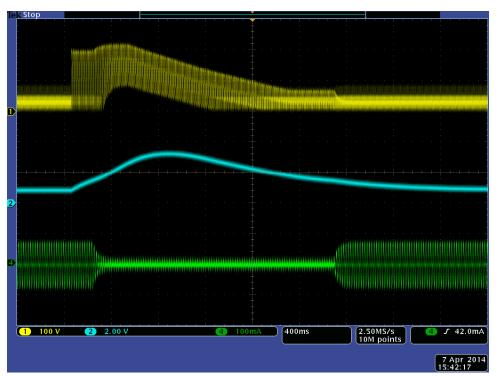
Figure 5. Drain Voltage (Top), DOV Pin Voltage (Middle), and Input Current (Bottom)
