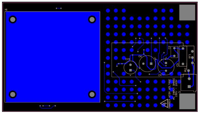
Figure 16. Bottom Layer and Bottom Overlay (Bottom View)
