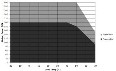
Convection load: 200 W up to 40 °C De-rate between 40-50 °C @ 1% per °C De-rate above 50 °C @ 2.5% per °C
