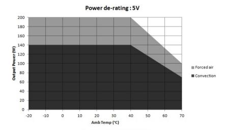
Convection load: 140 W up to 40 °C De-rate above 40 °C @ 1.67% per °C
