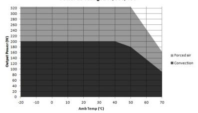
Convection load: 200 W up to 40 °C De-rate between 40-50 °C @ 1% per °C De-rate above 50 °C @ 2.5% per °C
