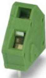
PCB terminal block, nominal current: 16 A, nom. voltage: 400 V, pitch: 5 mm, number of positions: 1, connection method: Spring-cage connection, mounting: Wave soldering, conductor/PCB connection direction: 45 °, color: red. End terminal block for terminating custom-grouped blocks.
