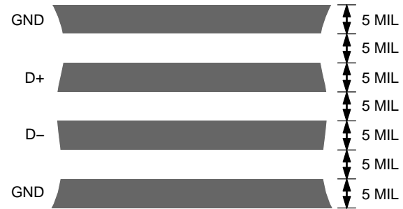
Figure 12. Typical Assignment of Signal Tracks
