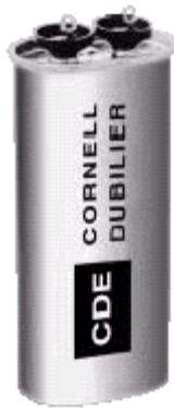
With a robust film/paper/extended foil construction, Type SNU capacitors have low inductance and high peak current ratings that make them ideal for power snubber applications. The Type SNU may be used to reduce voltage transients across semiconductor devices such as SCRs.
