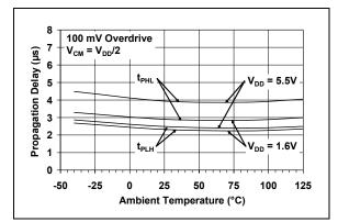
**FIGURE 2-29:** Propagation Delay vs. Ambient Temperature.
