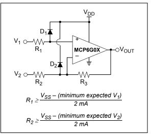
FIGURE 4-2: Protecting the Analog Inputs.
