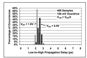
FIGURE 2-28: Low-to-High Propagation Delay.
