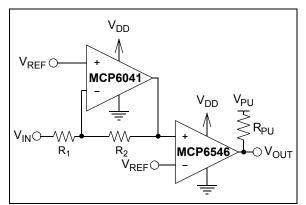
FIGURE 4-9: Precise Inverting Comparator.
