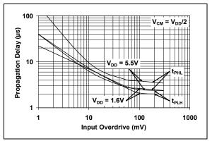
FIGURE 2-30: Propagation Delay vs. Input Overdrive.
