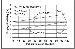
*FIGURE 2-32:* Propagation Delay vs. Pull-up Resistor.
