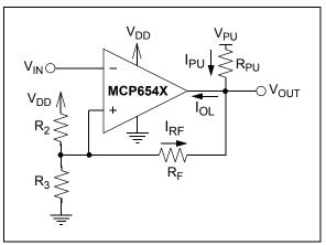
*FIGURE 4-4:* Inverting circuit with hysteresis.
