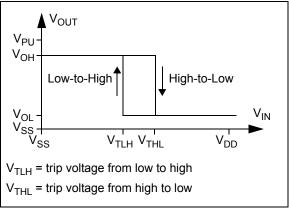
*FIGURE 4-5:* Hysteresis diagram for the inverting circuit.
