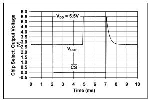
**FIGURE 2-39:** Chip Select  $\overline{(CS)}$  Step Response (MCP6548 only).
