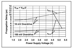
**FIGURE 2-27:** Propagation Delay vs. Power Supply Voltage.
