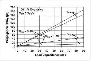
*FIGURE 2-35:* Propagation Delay vs. Load Capacitance.
