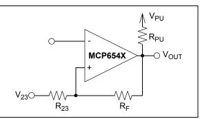
FIGURE 4-6: Thevenin Equivalent Circuit.
