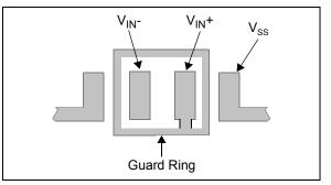
**FIGURE 4-7:** Example Guard Ring Layout for Inverting Circuit.
