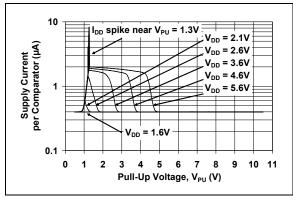
FIGURE 2-19: Supply Current vs. Pull-Up Voltage.
