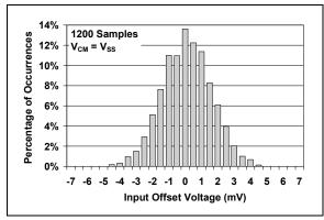
**FIGURE 2-1:** Input Offset Voltage at  $V_{CM} = V_{SS}$ .
