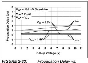
FIGURE 2-33: Pull-up Voltage.
