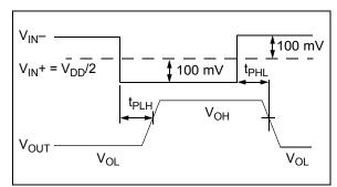
FIGURE 1-2: Propagation Delay Timing Diagram.
