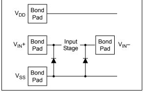
FIGURE 4-1: Simplified Analog Input ESD Structures.
