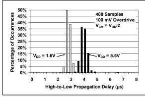
FIGURE 2-25: High-to-Low Propagation Delay.
