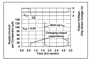
**FIGURE 2-41:** Supply Current (charging current) vs. Chip Select (CS) pulse at  $V_{DD}$  = 5.5V (MCP6548 only).
