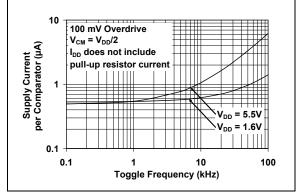
FIGURE 2-20: Supply Current vs. Toggle Frequency.
