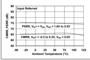
FIGURE 2-13: CMRR,PSRR vs. Ambient Temperature.
