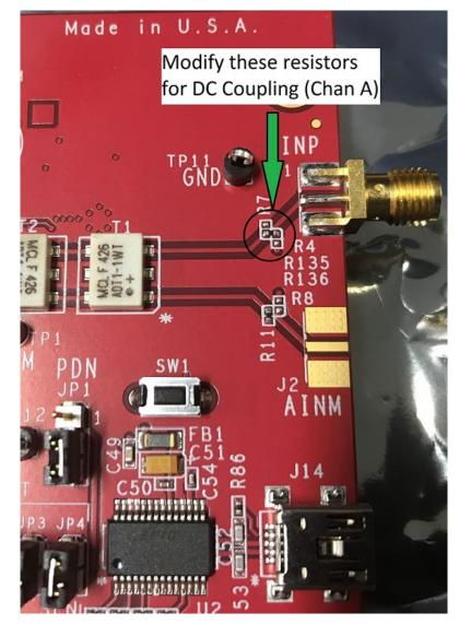
Figure 8. ADC32xxVM Input Coupling Configuration Resistors
