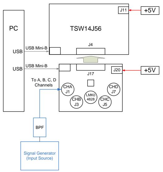
Figure 18. ADC32Jxx/ADC34Jxx and TSW14J56 Test Setup Block Diagram
