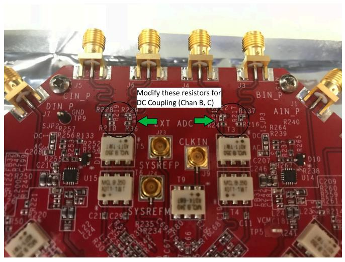
Figure 9. ADC3xJxx Input Coupling Configuration Resistors
