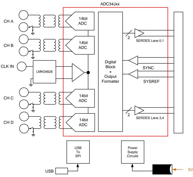
Figure 2. Simplified ADC34J4x EVM Block Diagram
