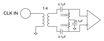
Figure 7. ADC34xx Clock Input Circuit
