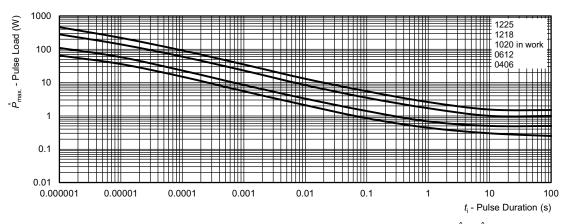
Maximum pulse load, single pulse; applicable if  $\bar{P} \to 0$  and n < 1000 and  $\ddot{U} \le \ddot{U}_{\text{max.}}$ ; for permissible resistance change equivalent to 8000 h operation
