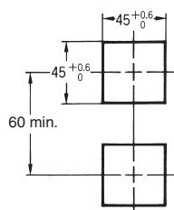
Side-by-side Mounting of N Controllers
