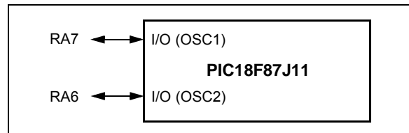
FIGURE 3-7: INTIO2 OSCILLATOR MODE
