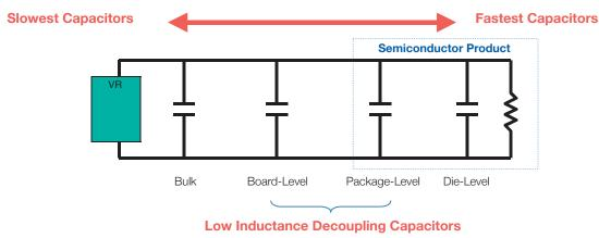
Figure 1 Classic Power Delivery Network (PDN) Architecture
