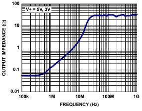
FIGURE 7. ENABLED OUTPUT IMPEDANCE vs FREQUENCY
