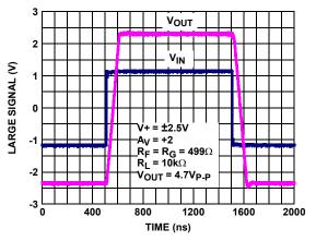
FIGURE 19. LARGE SIGNAL (4.7V) STEP RESPONSE
