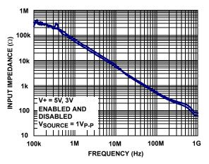
FIGURE 5. INPUT IMPEDANCE vs FREQUENCY
