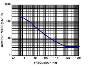
FIGURE 15. INPUT REFERRED NOISE CURRENT vs FREQUENCY
