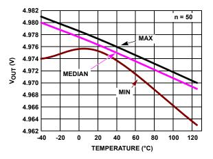
FIGURE 27. POSITIVE V<sub>OUT</sub> vs TEMPERATURE  $R_L = 1k$ ,  $V_S = \pm 2.5V$
