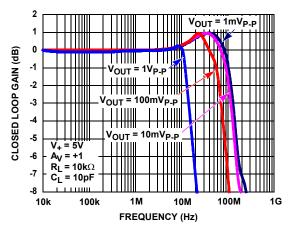
FIGURE 3. -3dB BANDWIDTH vs VOUT
