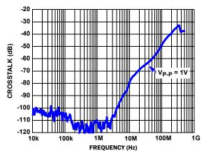
FIGURE 11. CHANNEL-TO-CHANNEL CROSSTALK vs FREQUENCY
