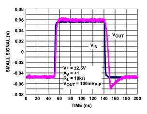
FIGURE 17. SMALL SIGNAL STEP RESPONSE
