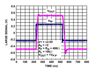
FIGURE 18. LARGE SIGNAL (1V) STEP RESPONSE
