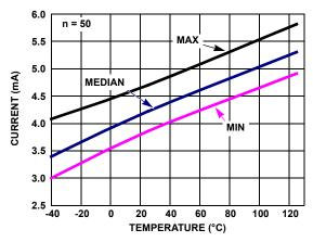
FIGURE 20. SUPPLY CURRENT vs TEMPERATURE, V<sub>S</sub> =  $\pm 2.5$ V ENABLED, R<sub>L</sub> = INF
