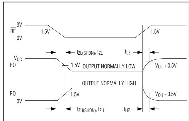
Figure 12. Receiver Enable and Disable Times (except MAX3081/MAX3084/MAX3087)
