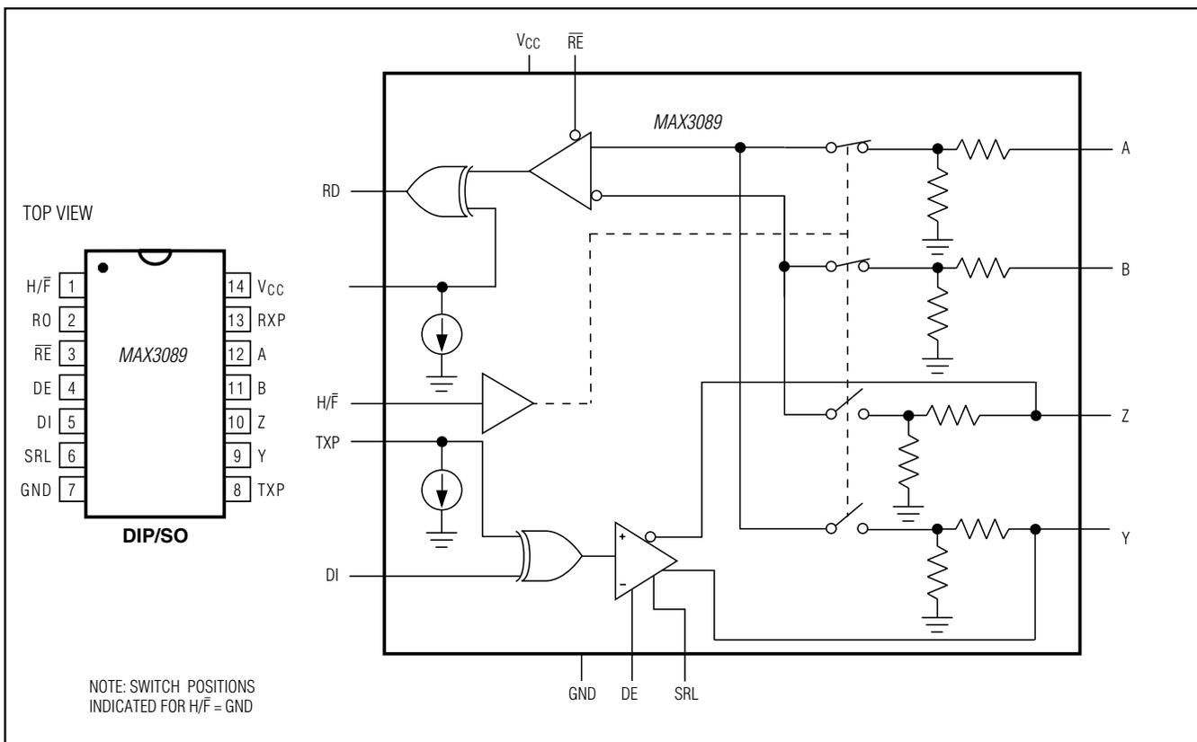
Figure 4. MAX3089 Pin Configuration and Functional Diagram
