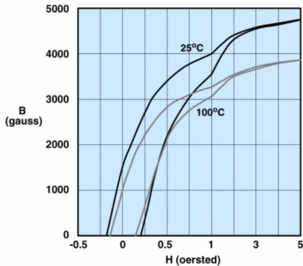
Measured on an 18/10/6mm toroid at 10kHz.
