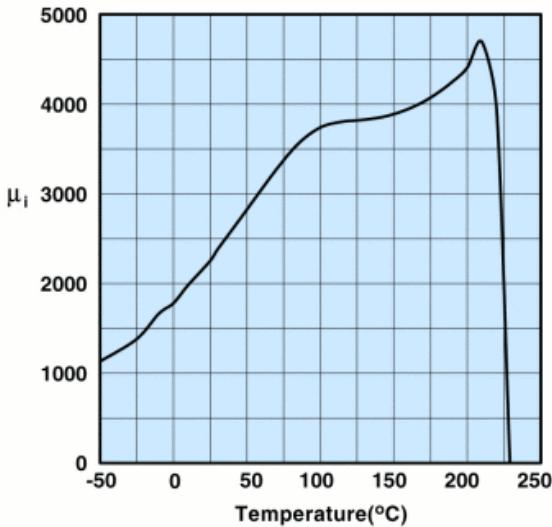
Measured on an 18/10/6mm toroid at 100kHz.
