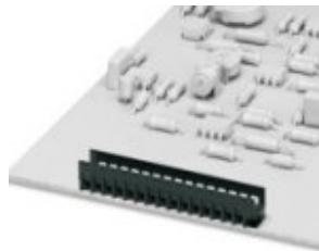
PCB headers, nominal current: 3 A, rated voltage (III/2): 250 V, number of positions: 7, pitch: 3.5 mm, color: black, contact surface: Tin, mounting: THR soldering, The touch-protected basic strip, serves to accommodate the FK-MPT 0,5 PCB terminal block.
