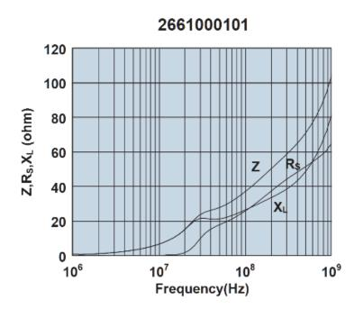
Impedance, reactance, and resistance vs. frequency.
