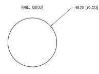
\*UNLESS OTHERWISE SPECIFIED TOLERANCES PER DECIMAL PRECISION ARE: X=±1 (±0.039), XX=±0.5 (±0.020), XXX=±0.25 (±0.010), XXXX=±0.127 (±0.005). LEAD SIZE=±0.05 (±0.002), LEAD LENGTH=±0.75 (±0.030). MIN=  $\frac{+DECIMAL}{-DECIMAL}$  PRECISION MAX.=  $\frac{+0.00}{-DECIMAL}$
