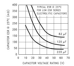
Figure 32. Capacitor ESR vs Capacitor Voltage Rating (Typical Low ESR Electrolytic Capacitor)
