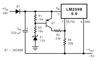
Figure 24. Undervoltage Lockout Without Hysteresis for an Inverting Regulator
