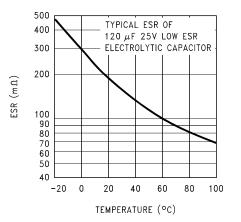
Figure 33. Capacitor ESR Change vs Temperature
