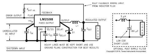
$\begin{array}{ll} \mbox{Component Values shown are for $V_{IN}$ = 15 V, $V_{OUT}$ = 5 V, $I_{LOAD}$ = 1 A. $120-\mu$F, 50-V, Aluminum Electrolytic Nichicon $PL$ Series $120-\mu$F, 35-V Aluminum Electrolytic, Nichicon $PL$ Series $3-A, 40-V $Schottky Rectifier, 1N5822 $ $8-\mu$H, $L30 $ $Typical Values $$^C_{SS}$ = 0.1 $\mu$F $$C_{DELAY}$: $-0.1 $\mu$F $$R_{Pull Up}$: $-4.7k$ $ \end{tabular}$
