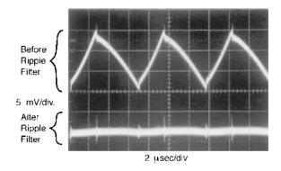
Figure 27. Post Ripple Filter Waveform
