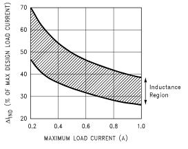
Figure 34. (∆I<sub>IND</sub>) Peak-to-Peak Inductor Ripple Current (as a Percentage of the Load Current) vs Load Current
