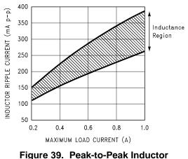
Ripple Current vs Load Current
