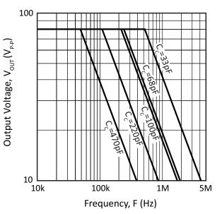
Figure 6: Small Signal Response w/ Boost
