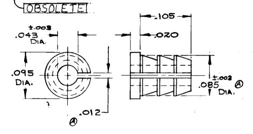
CONTRACT NO. UNLESS OTHERWISE AMP INCORPORATED SPECIFIED DIMENSIONS ARE IN INCHES HARRISBURG, PENNSYLVANIA TOLERANCES ON: DECIMALS ± .C ANGLES ± ± 005 NAME MATERIAL BUSHING, GROUND BRASS CODE IDENT NO. NUMBER DSGN APPD SIZE **(** 86280 00779 OTHER APPD SCALE SHEET
