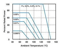
UPW Series resistors must be derated for tolerances below 0.1%. Use the graph to select tolerance versus operating temperature to determine the percentage rated power for operation.
