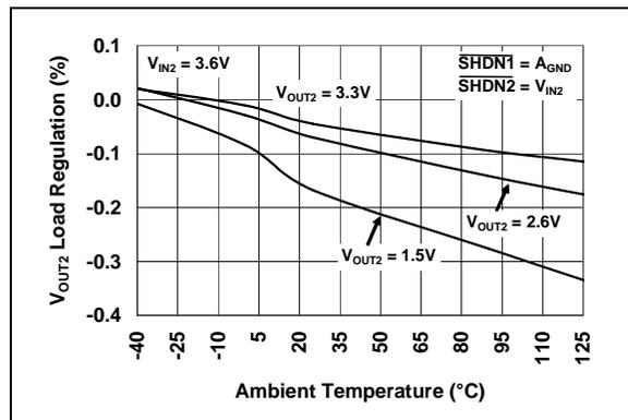
**FIGURE 2-29:**  $V_{OUT2}$  Load Regulation vs. Ambient Temperature.
