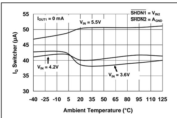
**FIGURE 2-3:**  $I_Q$  Switcher Current vs. Ambient Temperature.
