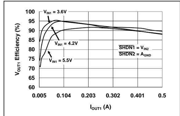
**FIGURE 2-10:**  $V_{OUT1}$  Output Efficiency vs.  $I_{OUT1}$  ( $V_{OUT1} = 3.3V$ ).
