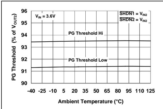
**FIGURE 2-31:** PG Threshold Voltage vs. Ambient Temperature.
