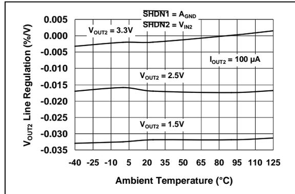
**FIGURE 2-28:**  $V_{OUT2}$  Line Regulation vs. Ambient Temperature.
