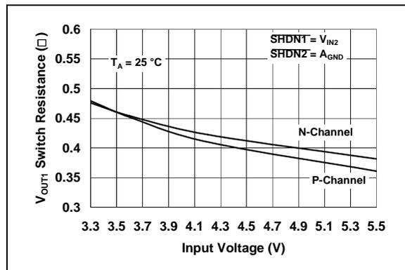
**FIGURE 2-17:**  $V_{OUT1}$  Switch Resistance vs. Input Voltage.
