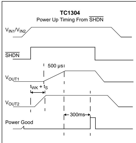
**FIGURE 4-3:** TC1304 Power-up Timing from  $\overline{\text{SHDN}}$ .
