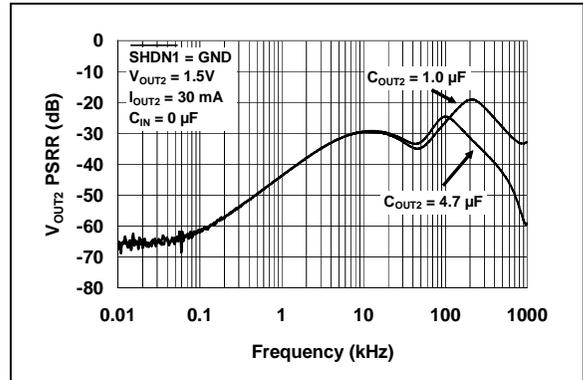
**FIGURE 2-34:**  $V_{OUT2}$  Power Supply Ripple Rejection vs. Frequency.
