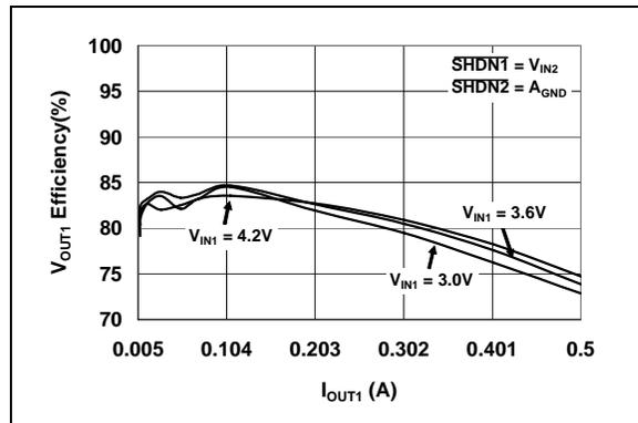
**FIGURE 2-6:**  $V_{OUT1}$  Output Efficiency vs.  $I_{OUT1}$  ( $V_{OUT1} = 1.2\text{V}$ ).
