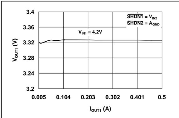
**FIGURE 2-13:**  $V_{OUT1}$  vs.  $I_{OUT1}$
