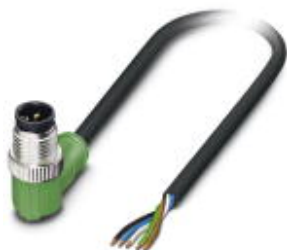
Sensor/actuator cable, 5-position, PVC, black RAL 9005, Plug angled M12, A - standard, on free cable end, cable length: 2 m
