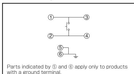
Parts indicated by ⑤ and ⑥ apply only to products with a ground terminal.
